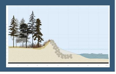
Rock revetment is a form of hard protection that involves the strategic placement of large rocks to provide protection from inundation and erosion. The rocks are placed on a slope and the irregular face of the rocks helps to dissipate wave energy.
