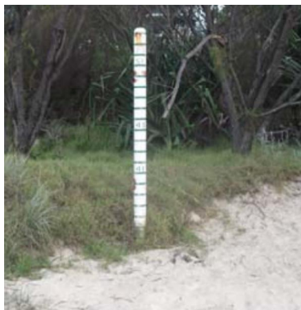
Figure 1: Example of a beach measuring pole from the COPE monitoring programme 3
