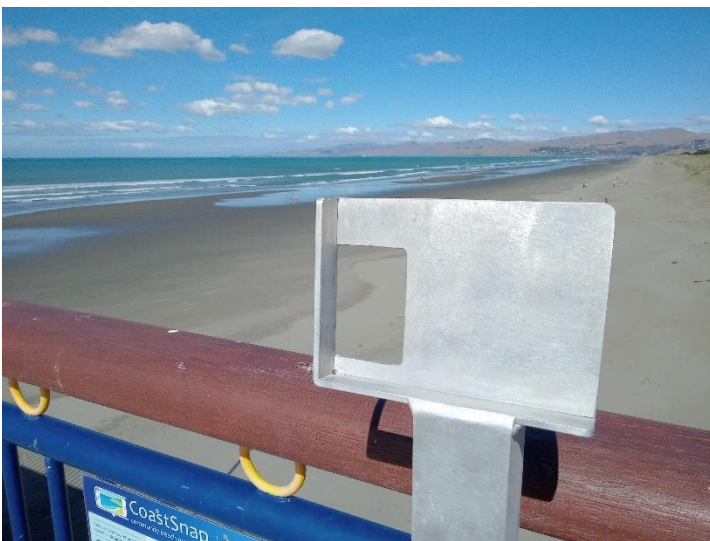
Figure 2: CoastSnap mobile cradle at the New Brighton Pier.
