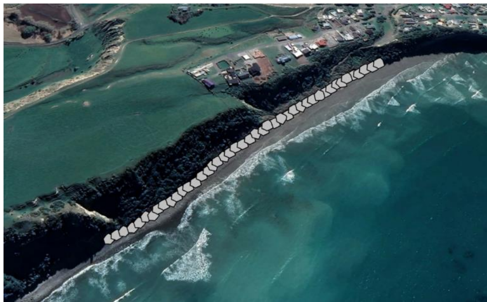
Figure 4.8: Approximate spatial location of the placement of rock along the toe of the cliff at Sandy Bay.
