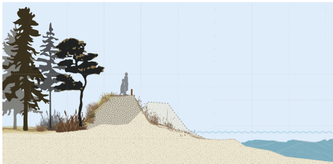
Figure 3.2: Conceptual sketch of total landward relocation of existing bund.
