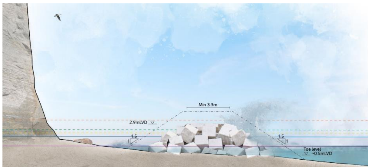
Figure 4.3: Conceptual diagram of a wave trip wall constructed from cast concrete blocks for a 30-year design life at the toe of the cliff.
