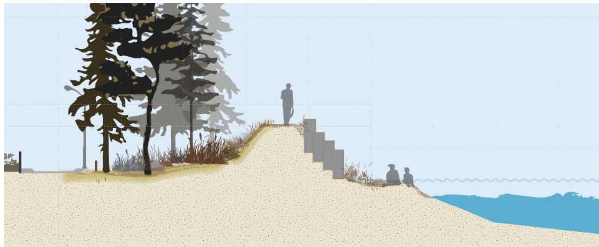
Figure 3.6: Conceptual sketch of the interlocking concrete wall option along existing bund alignment.
