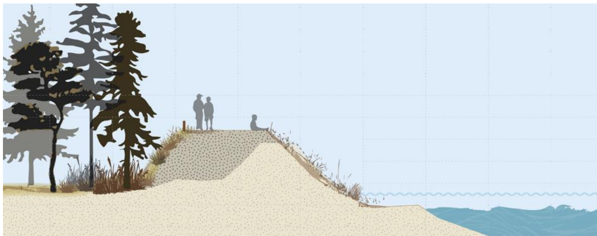
Figure 3.3: Conceptual sketch of the landward extension of the bund crest and increase in crest elevation.
