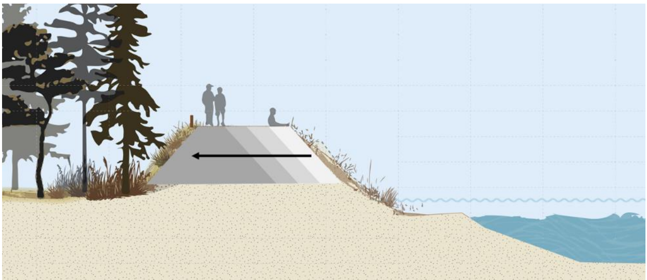
Figure 3.4: Conceptual sketch of the progressive relocation of the bund structure over a 10-30 year period, with the darker grey showing the bund footprint at the end of the consent period, 25 m landward of the existing bund structure.
