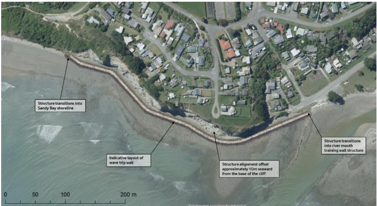
Figure 4.1: Proposed alignment of trip wall options.
