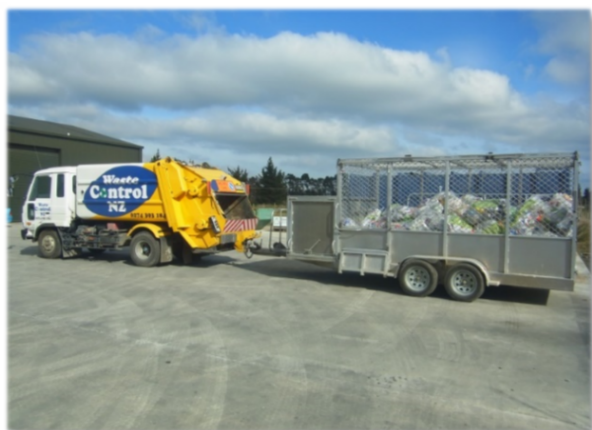
Kerbside refuse and recycling collection vehicle and trailer
