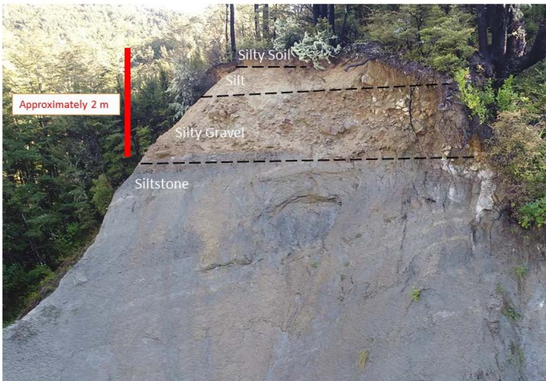
Figure 4: Typical stratigraphy at Mt Lyford Village. Photo taken at the south of Mt Lyford Village near Unnamed Stream.
