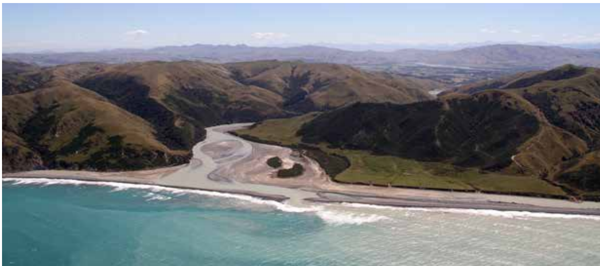
The Waiou River mouth, similar to other rivers in northern Canterbury, terminates in a hapua-type lagoon, created by sediment drift that builds up a beach barrier.
