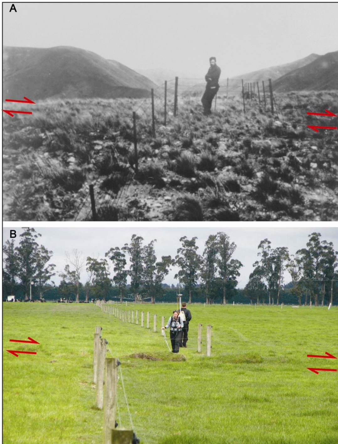
Figure 2 A: A fence offset sideways by ~2.4 m of strike-slip rupture on the Hope Fault at Glynn Wye during the 1888 North Canterbury Earthquake (Photo: A. McKay, GNS Science CN4852). B: A fence offset sideways by ~4.5 m of strike-slip rupture on the Greendale Fault during the 2010 Darfield Earthquake (Photo: N.J. Litchfield). Half-arrows either side of the fault indicate the direction of movement. In both cases, the movement is 'right-lateral', sometimes called 'dextral'. This means that to an observer, the ground on the far side of the fault has shifted sideways to the right. The effect is the same regardless of which side of the fault the observer is standing. The other type of strike-slip movement is 'left-lateral', sometimes called 'sinistral', but is not common in New Zealand.
