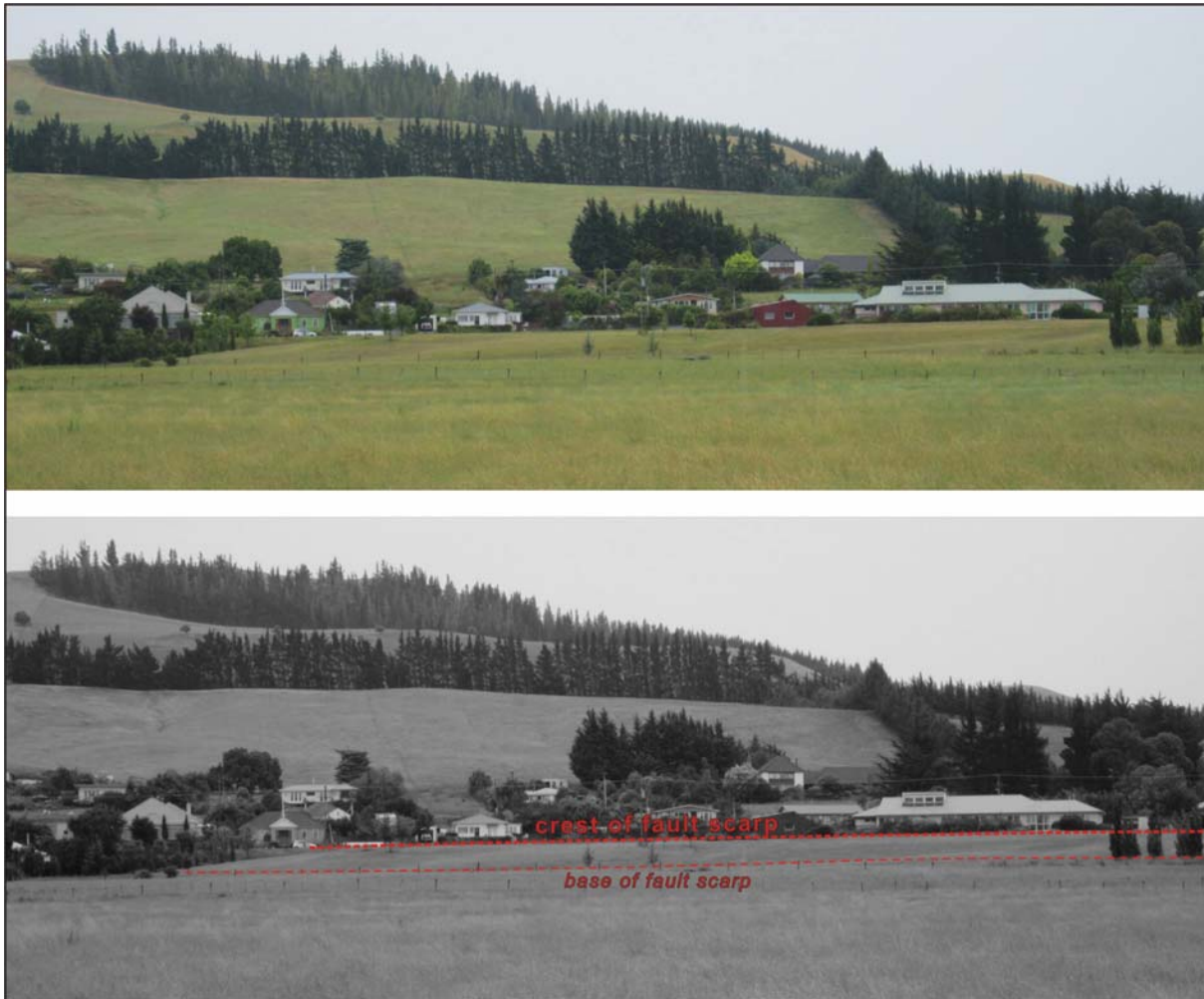
Figure 9 A view south from Kermode Street towards part of Waikari township, medical centre building on the right. The broad ~3 m high step running right-left in front of the buildings is thought likely to be a fault scarp, or possibly a monoclin flexure, associated with the Moores Hill Fault (Fig. 6, feature 27). A feature such as this could be investigated by trenching to establish whether it is in fact a fault, or of some other origin, such as a stream-trimmed terrace margin. Photo: D.J.A. Barrell.
