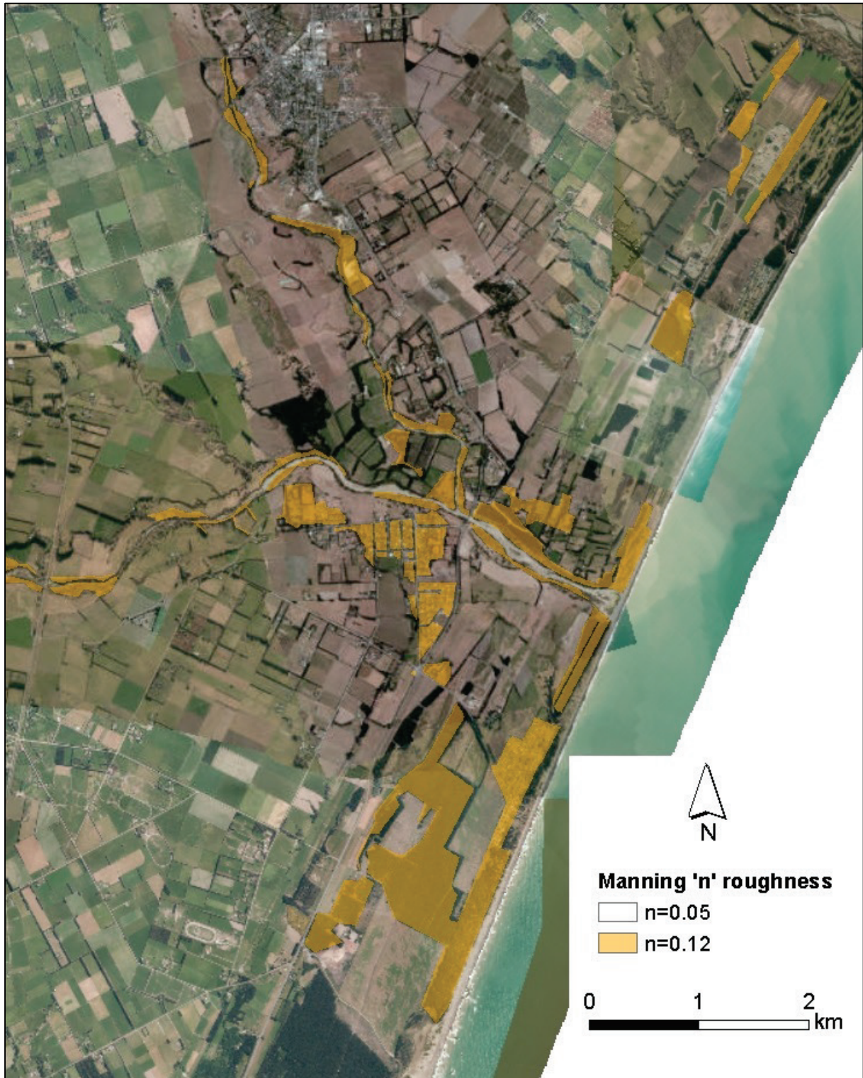
Figure D-4: Kowai River, Amberley Beach and Leithfield Beach floodplain roughness map showing Manning 'n'
