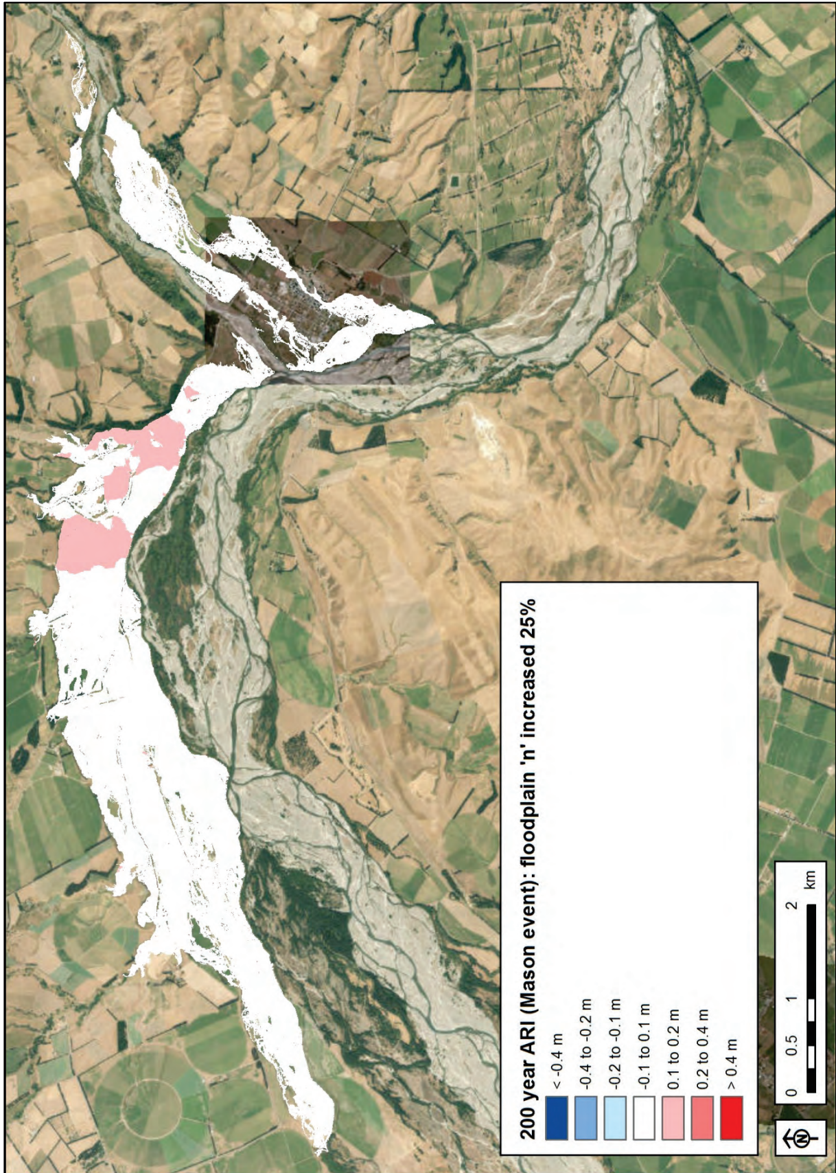
Figure 3-24: Change in maximum floodplain water depths when floodplain roughness is increased by 25% for the 200 year ARI Mason River flood event
