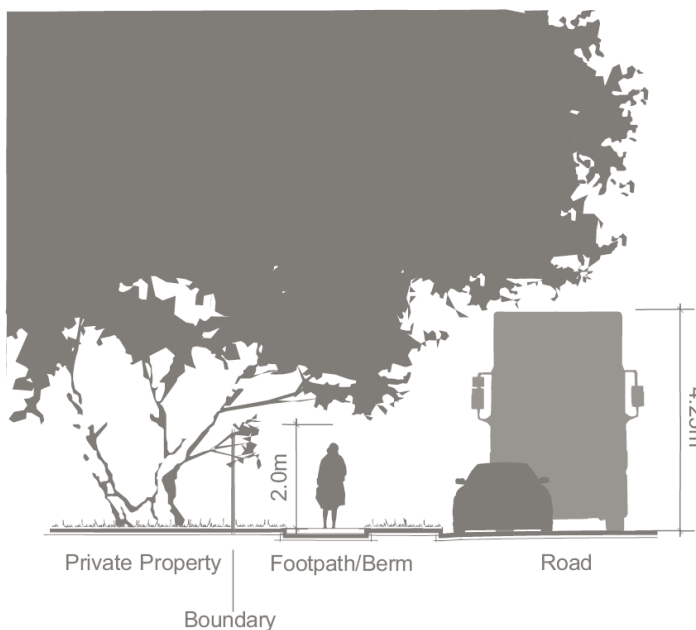
Figure 17 Private tree owner is required to maintain tree clearance over footpaths and road carriageways
